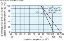
For resistors operated at an ambient temperature of 70°C or higher, the power (for RK73B, RK73H) or a current rating (for RK73Z) shall be derated in accordance with the above derating curve.
