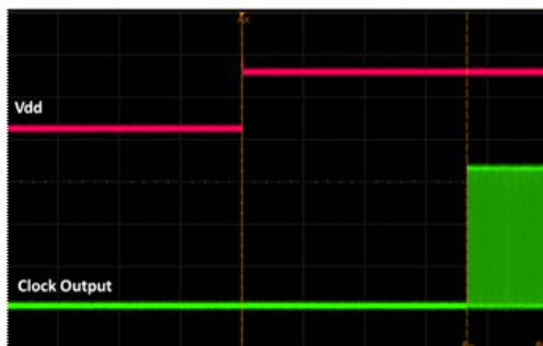
Figure 17. Startup Waveform vs. Vdd
