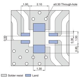
Coplanar waveguide(Line width and Gap of Line to GND) be designed to match 50\Omega characteristic impedance, depending on PCB material and thickness.
