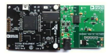
The **EVAL-CN0218-SDPZ** board monitors current in systems with high positive common-mode dc voltages of up to +500 V with less than 0.2% error. The load current passes through a shunt resistor, which is external to the circuit. The shunt resistor value is chosen so that the shunt voltage is approximately 500 mV at maximum load current. When using this evaluation board with the SDP board or BeMicro SDK board, apply +6 V and GND to Connector J2.
