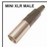
30-640-3 3 pin 30-640-4 4 pin 30-640-5 5 pin 30-640-6 6 pin Inline male MINI XLR plug. Also available with short boot. Cable opening .13"-.17"
