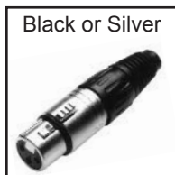
30-529-BK 30-529-SL XLR 3-pin male plug, twist-on strain relief. .15" to .3" cable opening. 4 piece construction. Internal compression style cable strain relief.
