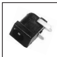
30-370-2.5 2.5 mm pin, 30-370-2.1 2.1 mm pin, PC mount coax power jack, switched circuit.
