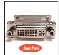
35-710 DVI-I to DVI-I Female to Female Coupler. Shielded di-cast case handles 5 pin analog and 24 pin digital signals. gold plated contact pins. Used for inline or chassis mount. Fits in standard DB15 d- sub cutout. Overall length .93" For wall mounting use Calrad p/n 30-598.
