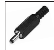
30-336 Coaxial power plug. 1.0mm I.D. 3.8mm O.D. .17" cable opening.
