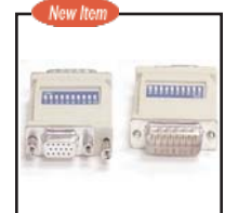
30-594 VGA to MAC adapter, 10 position Dip Switch For connecting Apple 15 pin D sub (2 rows) to 15 pin (3 rows) D sub connectors. Supports Apple standard display modes including 13" color (640x480) 16" (832x- 624) 21" (1152x870). Dip switch selectable for different display modes.
