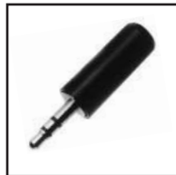
30-489 3.5 mm dia., stereo Audio Plug with plastic handle. No Strain relief .21" cable opening.
