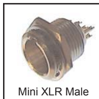
30-642-3 3 pin 30-642-4 4 pin 30-642-5 5 pin 30-642-6 6 pin Chassis mount MINI XLR male. Mounts in .43" "D" hole. Nickel plated body.
