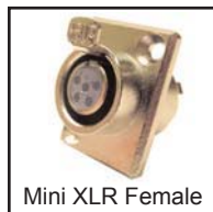
30-643-3 3 pin 30-643-4 4 pin 30-643-5 5 pin 30-643-6 6 pin Chassis mount MINI female XLR. Mounts in 15.20mm, .60 hole. Nickel plated body.
