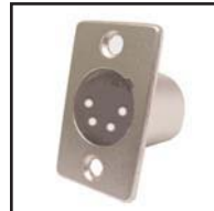
30-522-SL-4 4-pin male XLR chassis plug mounts in .75" hole size.
