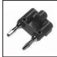
30-440 Red 30-441 Black Dual banana plug, gold plated. .24" cable opening. 0.75" centers.
