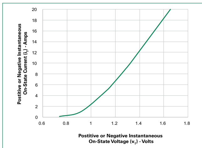
Figure 7: On-State Current vs. On-State Voltage (Typical)
