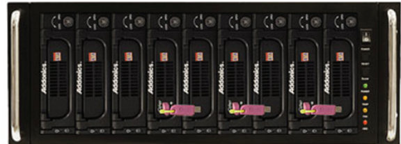
Storage Rack with 9x Mobile Rack
