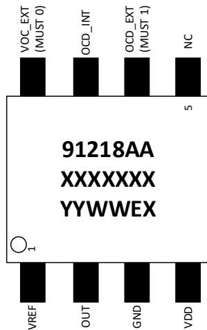
Figure 12: SOIC8 - Pinout and marking
