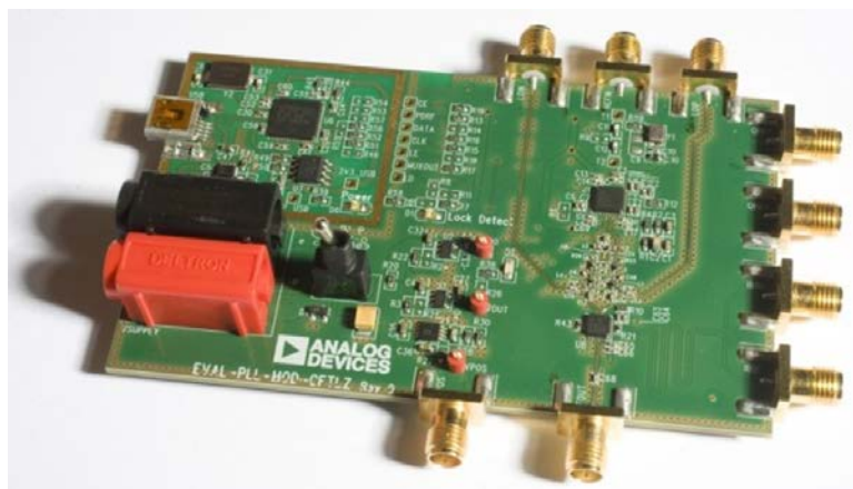
Figure 2. Evaluation Board for CN-0285 Direct Conversion Transmitter
