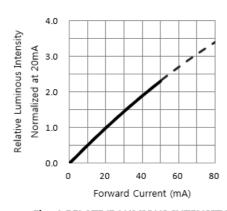
Fig. 4 RELATIVE LUMIOUS INTENSITY VS. FORWARD CURRENT
