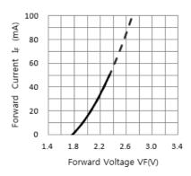
Fig. 2 FORWARD CURRENT VS. FORWARD VOLTAGE
