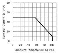
Fig. 3 FORWARD CURRENT VS. DERATING CURVE
