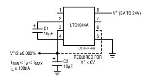
Figure 8. Ultra-Precision Voltage Divider
