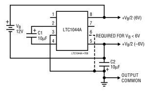
Figure 9. Battery Splitter
