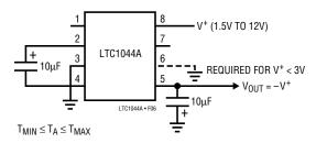
Figure 6. Negative Voltage Converter
