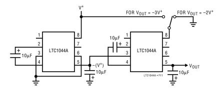
Figure 11. Stacking for Higher Voltage
