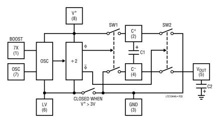
Figure 3. LTC1044A Switched-Capacitor Voltage Converter Block Diagram
