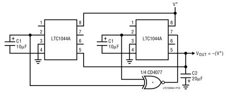
\*THE EXCLUSIVE NOR GATE SYNCHRONIZES BOTH LTC1044As TO MINIMIZE RIPPLE
