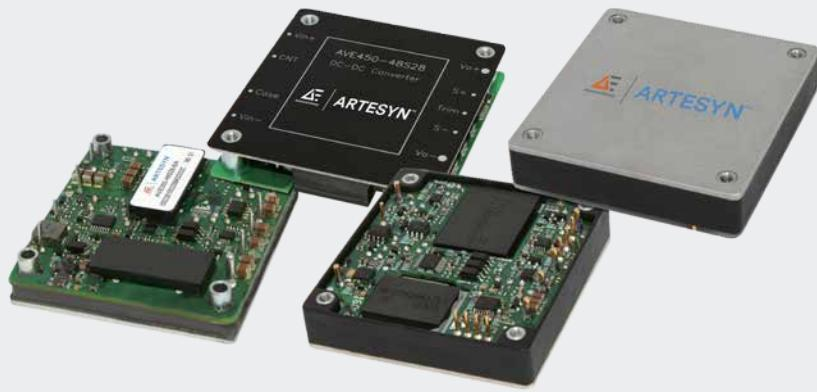
Advanced Energy's Artesyn AVE450/500 series half-brick isolated DC-DC converter provides a single regulated low noise output, 28 Vdc that can deliver up to 16 amps (AVE450B-48S28) or 50V that can deliver up to 10 amps (AVE500-48S50). It has a wide 2:1 input range of 36 to 75 Vdc and is designed primarily for use with standard 48 V telecommunications equipment supplies. The converter's main application area is in low power and remote radio head (RRH) telecommunications applications.
