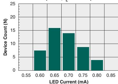
**Typical  $I_F$  for Switch Dropout
