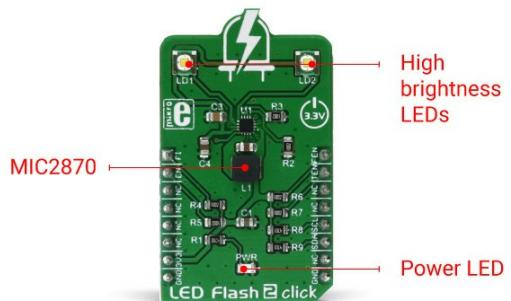
Flash inhibition pin, or the FI pin - routed to the mikroBUS™ AN pin, with the corresponding bit in the Torch control register (02h), is used to limit the Flash mode current value to the Torch mode current value. This will effectively override the Flash mode.
