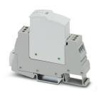
Type 2/3 surge protection, consisting of protective plug and base element with screw connection. For single-phase power supply network with integrated status indicator and remote signaling. Nominal voltage: 230 V AC/DC
