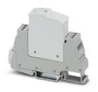
Type 2/3 surge protection, consisting of protective plug and base element, with integrated status indicator and remote signaling for single-phase power supply networks. Nominal voltage: 120 V AC/DC
