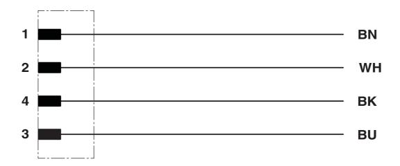
Contact assignment of the M8 plug
