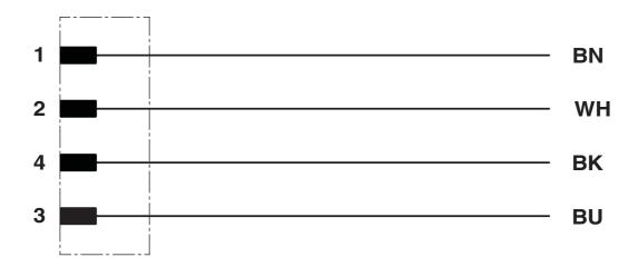
Contact assignment of the M12 plug
