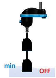
Low level stops the pump
