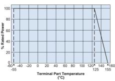
For resistors operated terminal temperature of described for each size or above, a power rating shall be derated in accordance with the derating curve. Please refer to "Introduction of the derating curve based on the terminal part temperature" in the beginning of our catalog before use.
