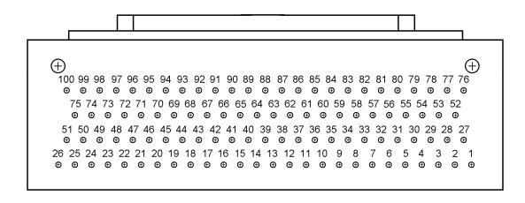
NOTE: Engaging face of socket insert shown, cavity identification numbers are for reference only and do not appear on the part.
