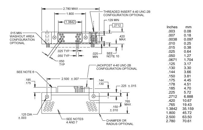
FIGURE 1. Connector, receptacle, .050 inch (1.27mm) spacing.
