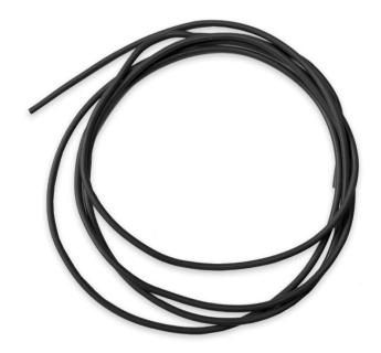
Mueller's WI-M-10-@ is 10 AWG, 1050/0.08 stranded, tinned copper wire with highly flexible 0.197" (5mm) diameter silicone jacket.
