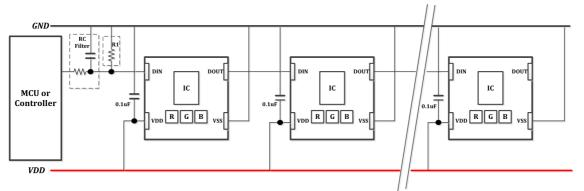
Cascading connection for normal driver IC embedded LEDs is shown. The data signal is transmitted one-by-one. The output of the previous one is connected to the input of the next one. As for the power positive and negative, all LED positives should be connected to VDD and all LED negatives should be connected to ground.
