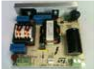
EVL6564-100W 100 W transition-mode PFC pre-regulator
