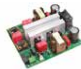
EVL4986A-1KWBL Low THD-High efficiency, 1 KW bridgeless CCM-PFC
