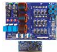
STDES-PFCBIDIR 15 kW, three-phase, three-level active front-end (AFE) bidirectional converter
