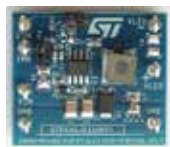
STEVAL-ILL056V1 3 A Buck LED driver board based on the LED5000
