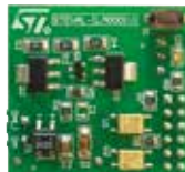
STEVAL-ILM001V1 Plug-in hardware module for the STM8S-DISCOVERY interface for DALI communication
