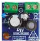
STEVAL-VP12201B 15 V/200 mA buck converter
