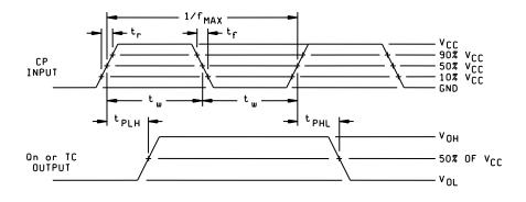
FIGURE 4. Switching waveforms and test circuit.
