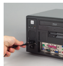
Plug ring-lock securely fastens the power cord
