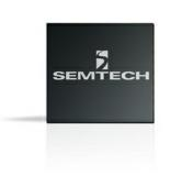
The GS6080 is a high-speed BiCMOS integrated circuit designed to drive one or two 75 Ohms coaxial cables. The GS6080 may drive data rates up to 5.94Gb/s and provides two selectable slew rates in order to achieve compliance to SMPTE ST 424, SMPTE ST 292 and SMPTE ST 259.
