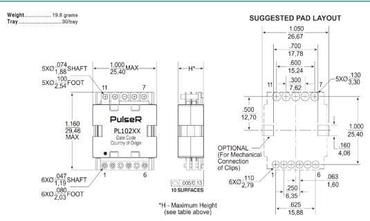
NOTE: The above is a universal footprint for a component that has all 11 pins populated. For a given part number it is only necessary to provide pads for the terminations shown
