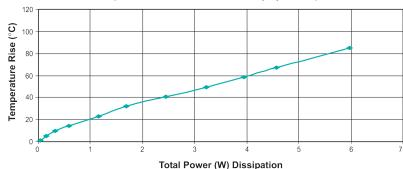
Total Power Dissipation (W) = .001 \* (DCRprimary \* IRMs\_primary2 + DCRsecondary \* IRMs\_secondary2) + Core Loss (W)
