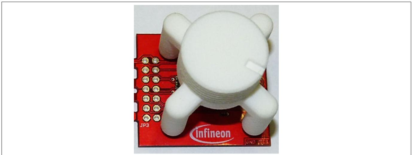
**Figure 2** Rotation knob with TLE5x09A16(D) angle sensor below
