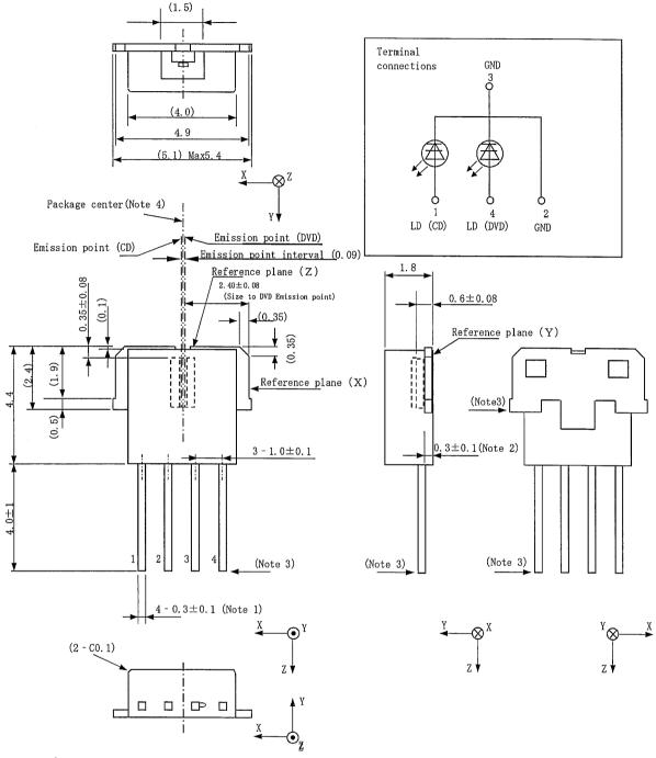
Note 1) Dimension of the bottom of lead pins.
