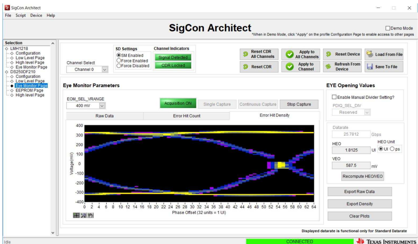
Figure 7. Eye Monitor Page for DS250DF230 Profile
