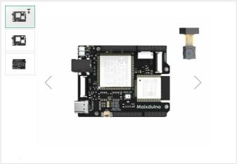
$Based \ on \ MAIX \ Module, the \ Maix duino \ is \ a \ RISC-V \ 64 \ development \ board \ for \ AI+IoT \ applications. \ Different \ with$ other Sipeed MAIX dev. boards, Maixduino was designed in an Arduino Uno form factor, with ESP32 module on board together with MAIX AI module.
