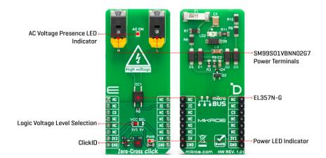
The current passes through the Graetz bridge circuitry, consisting of four DLGL5980. The alternate current converts to a direct current, which is necessary for driving an LED in an <u>EL357N-G</u>, a phototransistor photocoupler from Everlight. When activated, the optocoupler sends a LOW logic state to a ZC pin, which is the pin with which the Zero-Cross Click communicates with the host MCU.
