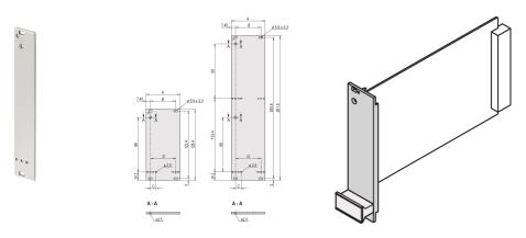
The front panel enables the assembly of a plastic or Alu-profile static trapezoid handle. The front panel cannot be shielded with a textile gasket.
