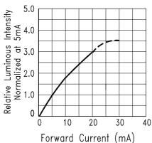
Fig.4 Relative Luminous Intensity vs. Forward Current
