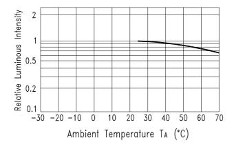
Fig.5 Luminous Intensity vs. Ambient Temperature
