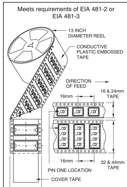
Each reel has a 15.750 inch (390 mm) minimum leader and a 6.30 inch (160 mm) minimum trailer.
