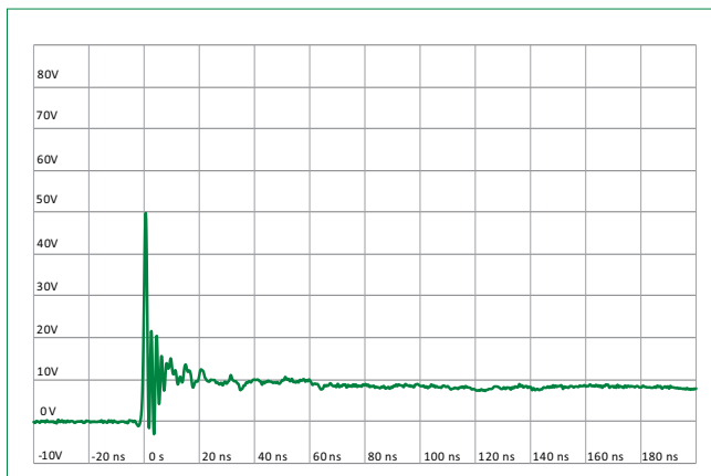
IEC 61000-4-2 +8 kV Contact ESD Clamping Voltage
