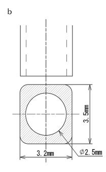
Nozzle with chamfering is recommended
