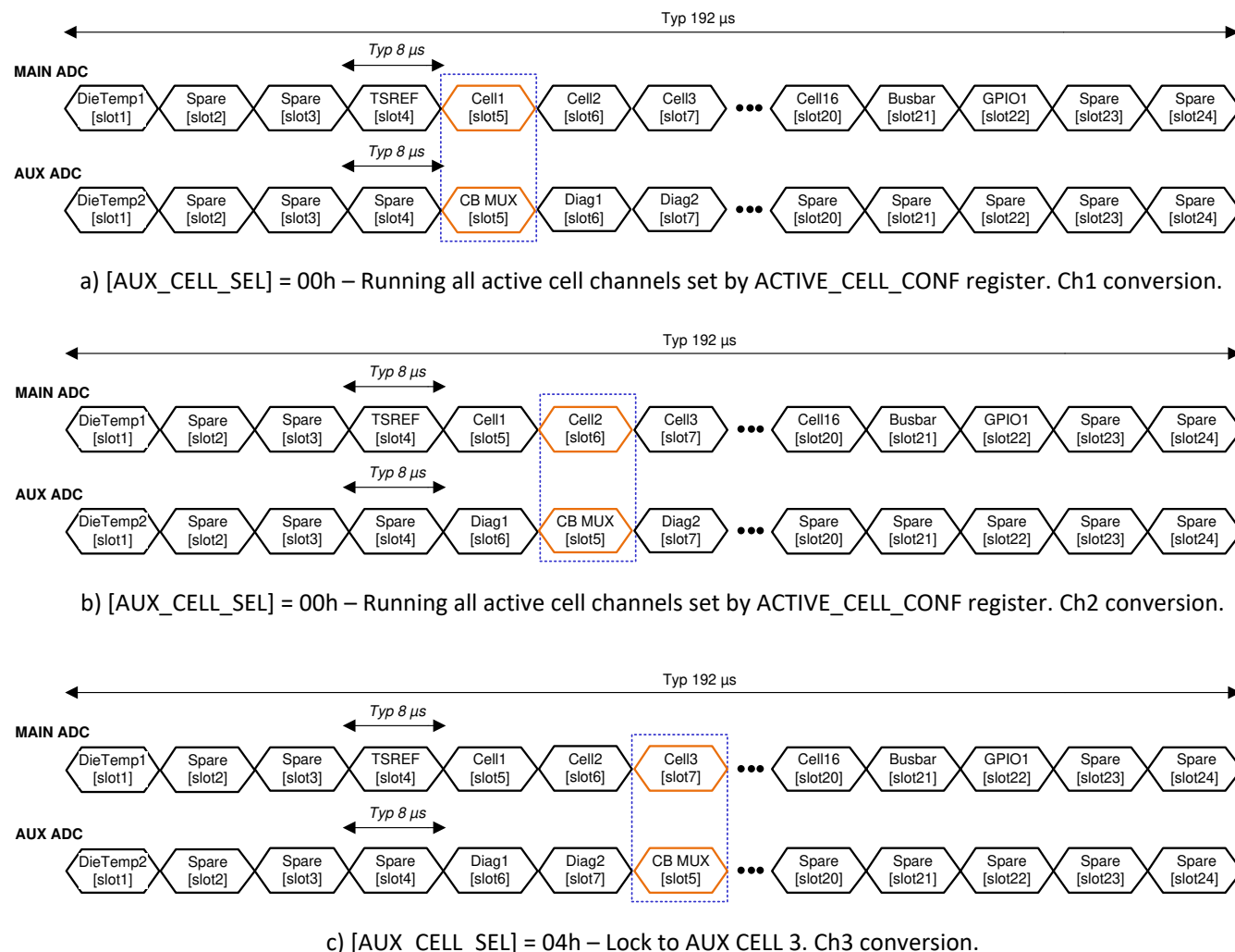
Figure 8-12. Synchronization Between MAIN and AUX ADC Sampling
