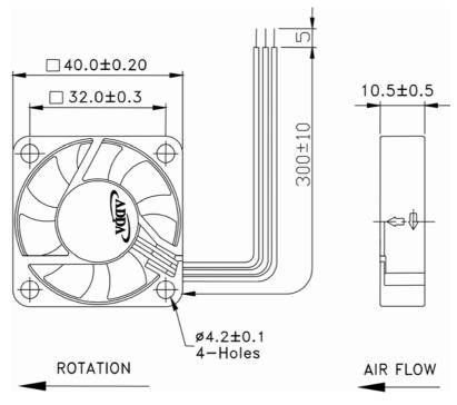
LEAD WIRES: UL 1007, AWG26, L = 300 +/- 10 mm Red = positive; Black = negative.
