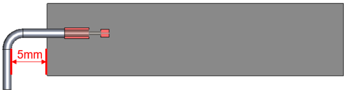
Figure 1 Cable Bending
