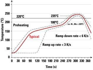
Note: Up to 2 reflow cycles in accordance with the above temperature profile
