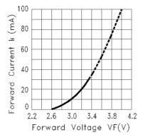
Fig.2 FORWARD CURRENT VS. FORWARD VOLTAGE
