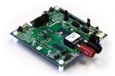
Agora application development requires the use of the Flidor development interface board. Flidor is a programmer, debugger, and breakout interface for Tectonic Edge™ compatible target devices deisgned by Embedded Planet such as Agora. Flidor provides adjustible power to the target MCU and connects it to a computer via USB for debugging in addition to its breakout capabilities.
