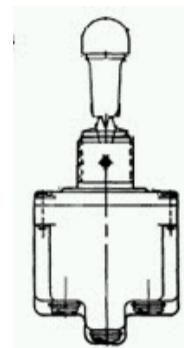
**TL Series Toggle Switch, 4 pole, 3 position, Screw terminal, Locking Lever**
