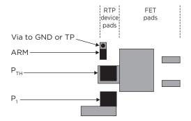
**Note:** Thermal conductivity between the RTP device and the heat source is highly dependent on board layout, heat sink structures, and relative placement and design of co-located components. It is the responsibility of the user to verify that the RTP device provides sufficient protection in the user's specific final device implementation.
