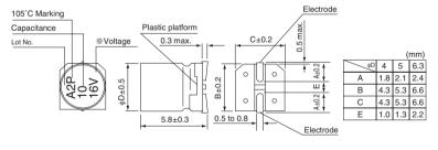
$\%\,\text{Voltage}$  mark for 6.3V is  $\,\lceil 6\text{V} \rfloor$
