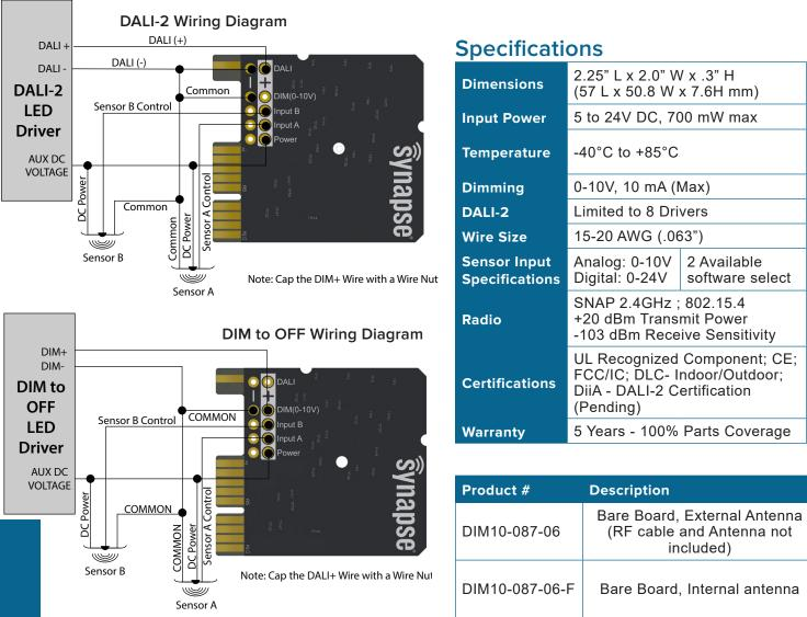
Note: Deployment is for inside fixtures only. Do NOT use in a fixture to fixture design.
