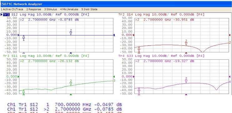
Ch1 Tr2 514 700.00000 MHz -33.458 Ch1 Tr2 514 2.7000000 GHz -30.951 dB Ch1 Tr3 S11 700.00000 MHZ -38.057 Tr3 511 2.7000000 GHz -26.132 Ch1 dB Tr4 533 700.00000 MHz -32.191 dB Ch1 Ch1 Tr4 533 2.7000000 GHz -19.327
