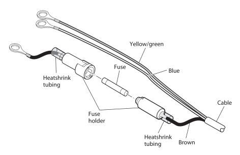
**Fuse Holder Installation:** This illustration shows where to install the fuse holder.
