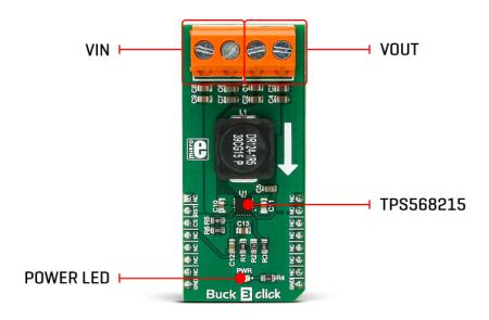
The onboard voltage divider connected to the MODE pin of the IC is used to set the device to work with the fixed PWM frequency of 800kHz, DCM/Eco-mode™ for light loads, and to set the limiting current to about 7A.
